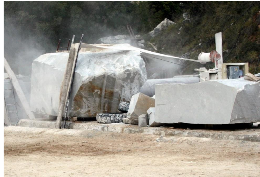
Rope saw for cutting marble
